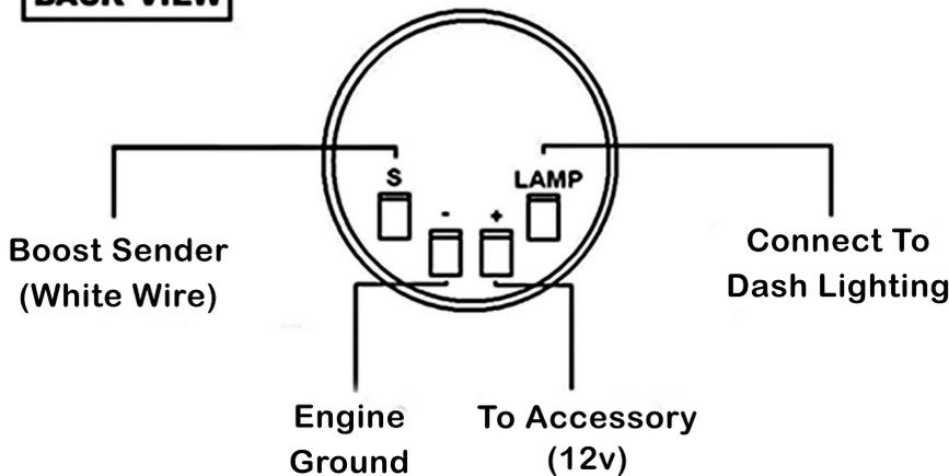
Cut boost line and install supplied plastic "T" fitting. Connect "T" fitting to the in-line filter with supplied hose. Then connect in-line filter to sender with supplied hose.
