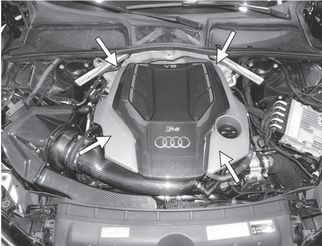
41) Reinstall the engine cover by pressing the cover down onto the four mounting posts on the engine.
