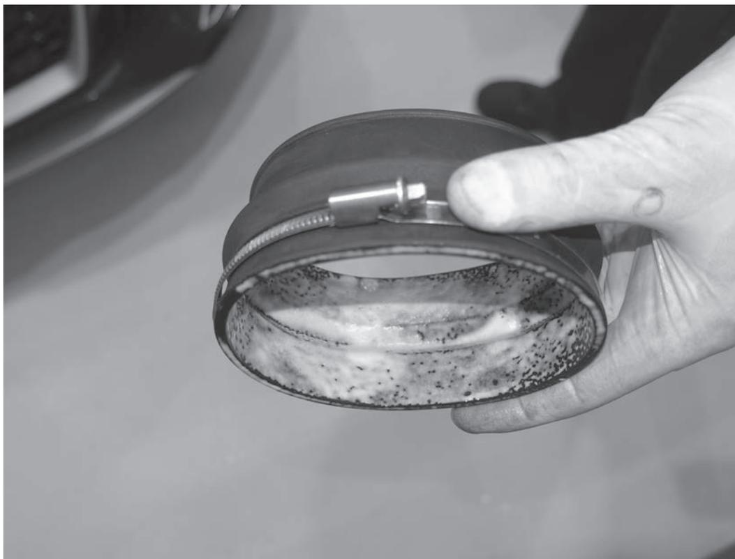
25) Generously lubricate the large APR coupler with one of the hose clamps. A foaming glass cleaner works well for this, and does not leave any residue.
