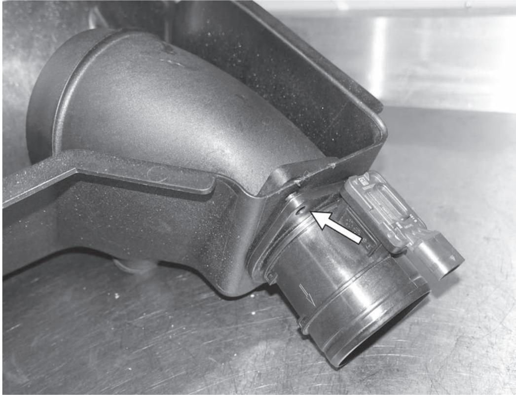
15) Place the MAF sensor or the APR MAF adapter into the back of the APR heat shield. Orient and install the APR filter adapter onto the MAF sensor from the other side of the heat shield.
