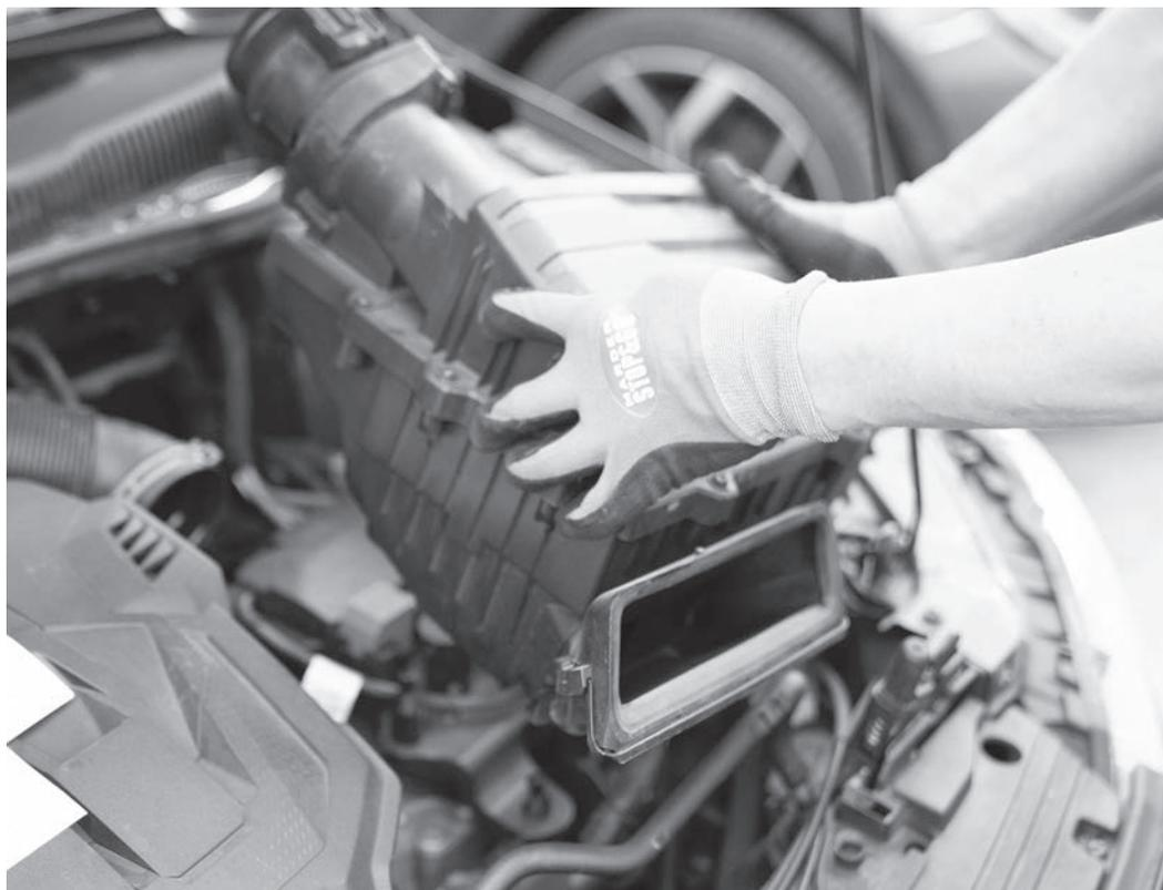
5) Lift the airbox assembly up and out of the car, separating it from the mounting posts underneath.
