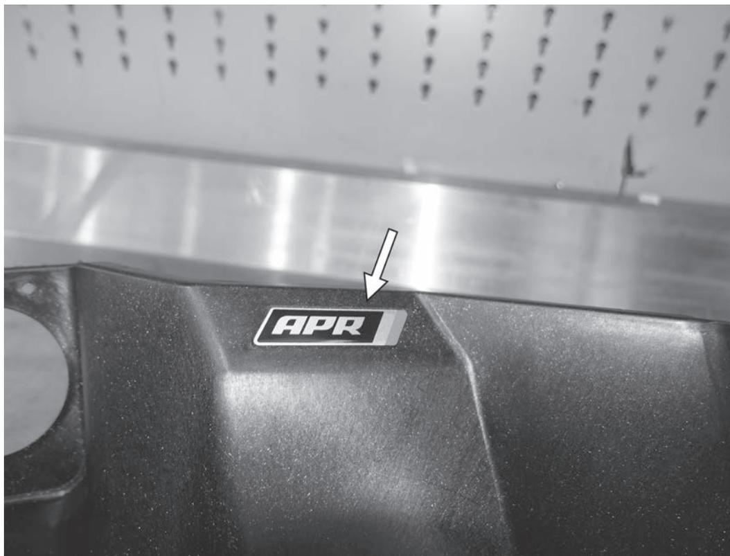
7) After removing the adhesive backing, place the APR logo in the recessed location on the top of the back of the APR heat shield.
