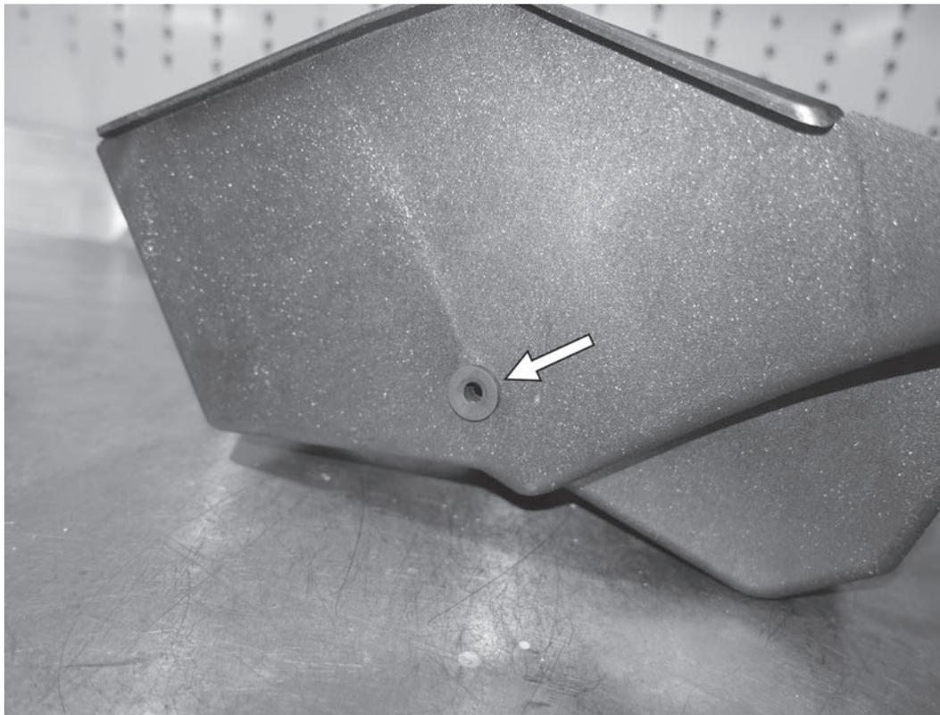
9) Using an evaporating lubricant, install the bigger of the two smaller rubber grommets into the side of the APR heat shield.
