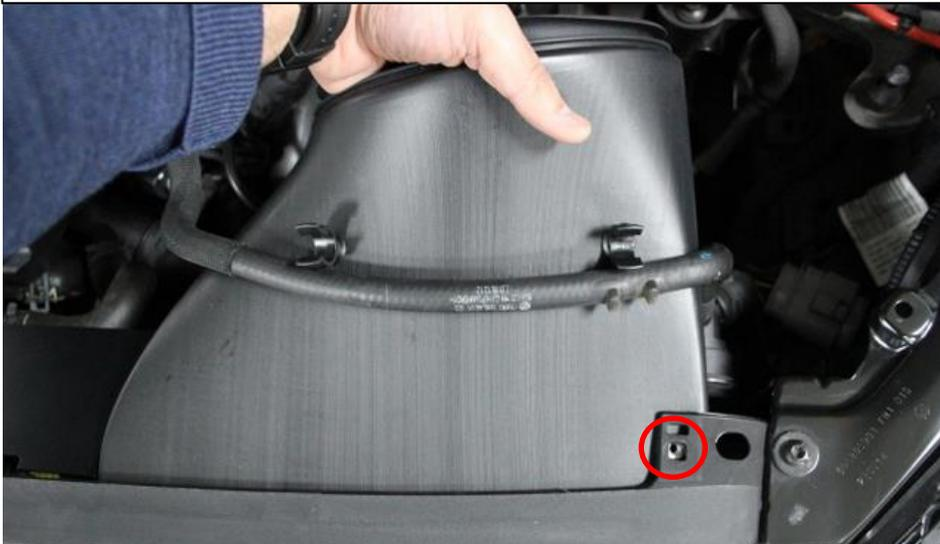
11. push the duct into place so that the securing nut on the duct lines up with the hole on the slam panel.
