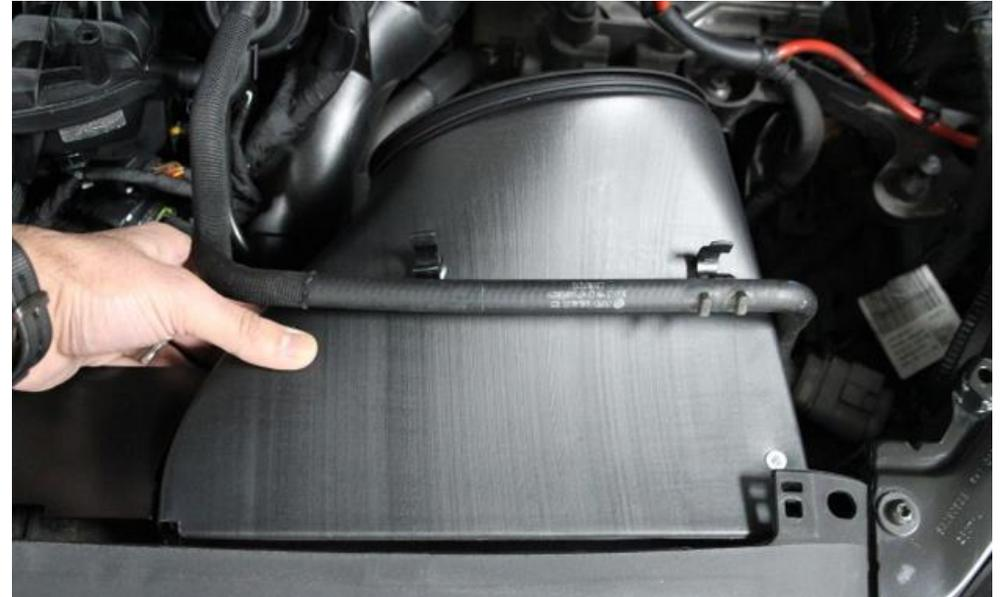
10. Place the duct assembly as shown and guide it into place – you might need to push the duct panels into place by inserting your hand inside the duct as shown in next step.
