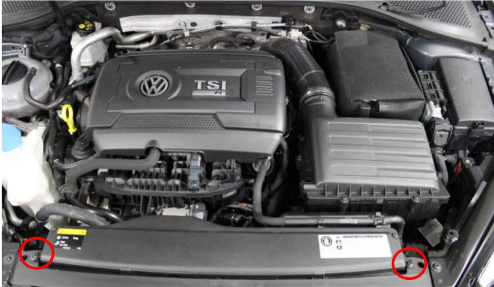
1. We will start by removing the stock airbox system. Remove the 2 screws holding the duct in place as shown.
