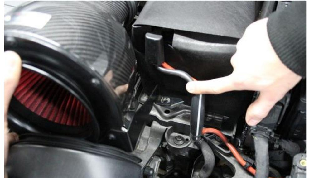
18. Lower the housing – push the battery cables away to allow the bracket to lower into position.
