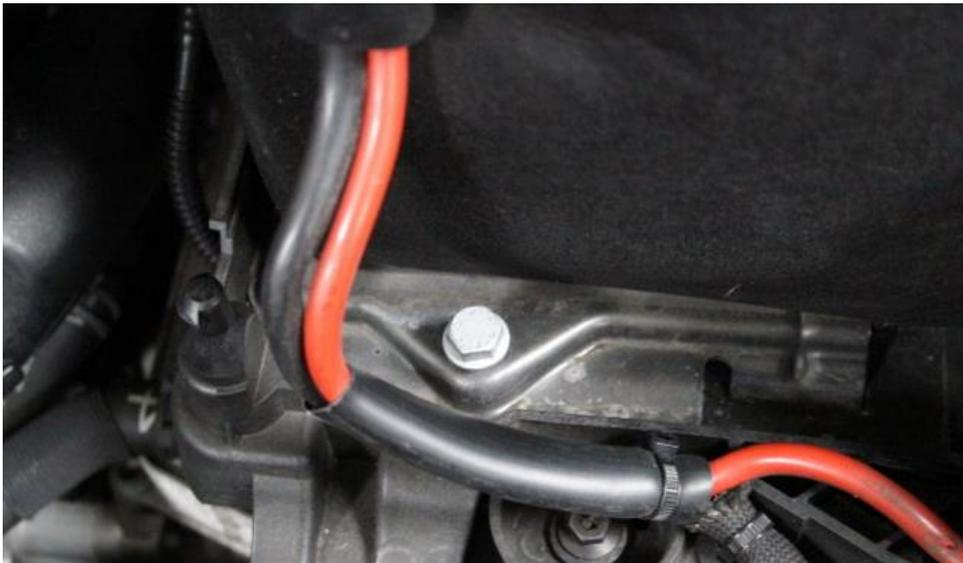
7. Remove this 13mm Bolt from the battery clamp. This is where the intake will secure.
