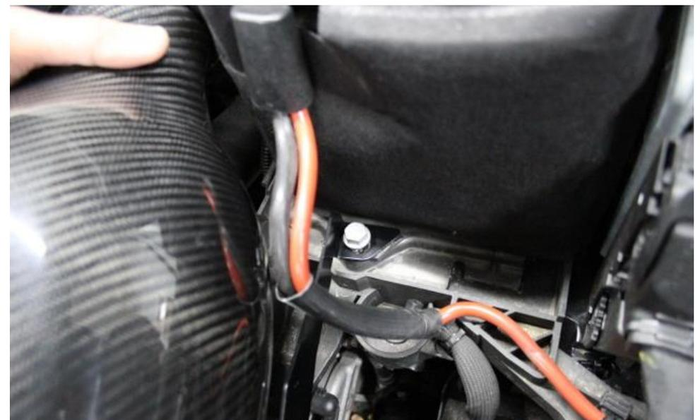
20. Keep the housing pressed against the duct and secure the bracket with the 13mm bolt removed in step 7.
