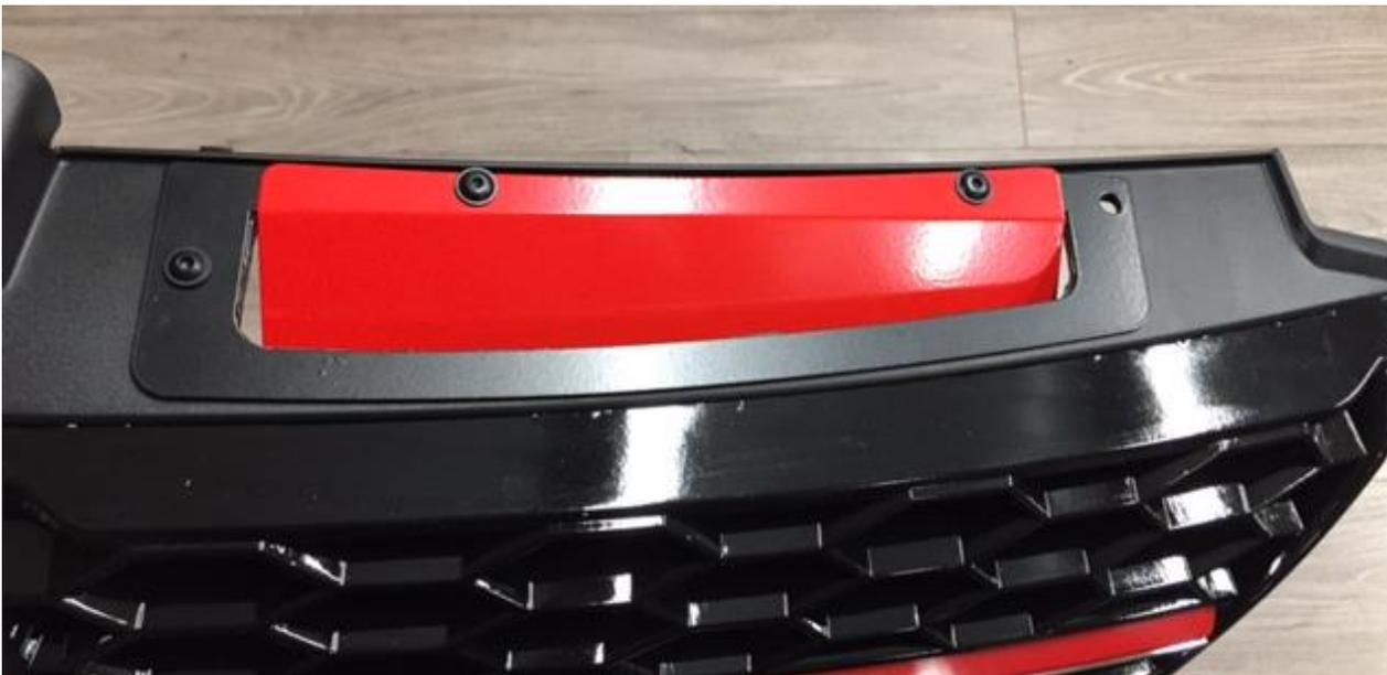
32. Now take the scoop and insert into the grill. Secure with 2 M5 screws and lock nuts.
