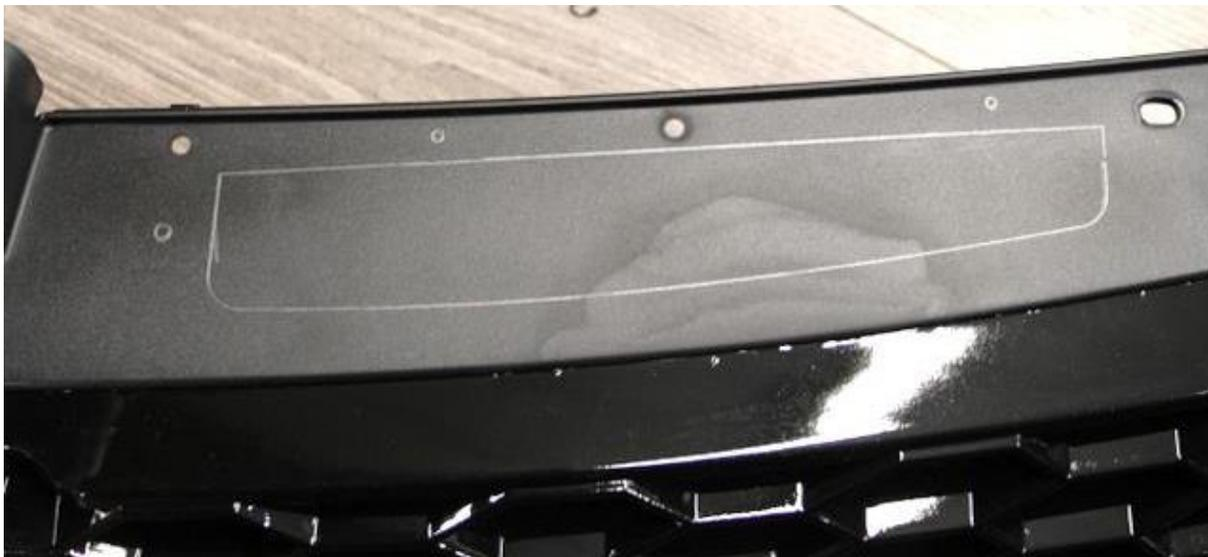
28. Carefully draw around the inside of the surround including the 3 remaining holes. We will use the supplied tool to cut the plastic.
