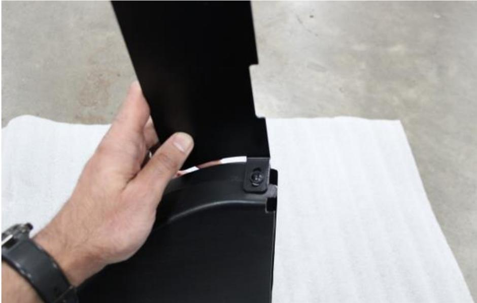
9. Using 1 supplied M5 screw, assemble the duct and panel as shown. Do not tighten this yet, we will need to adjust after installation.
