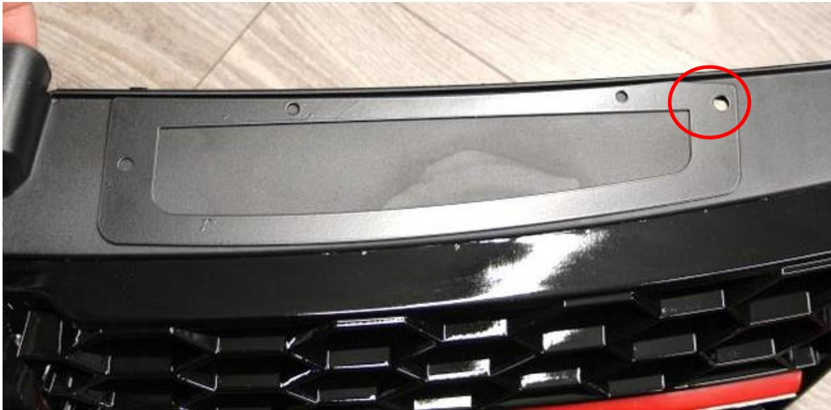
27. Now place the scoop surround panel on the grill – on the right side. Line up the hole on the right with the hole already in the grill. The rear edge of the panel should also meet the rear lip of the grill.
