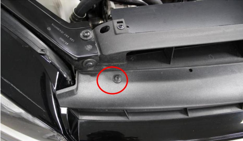
23. We will now remove the front grill. Start by removing the 2 screws, one on each side as shown here.
