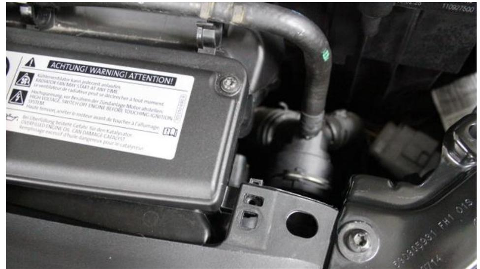
2. Now push the duct clips down to release from the slam panel. Do for both sides.
