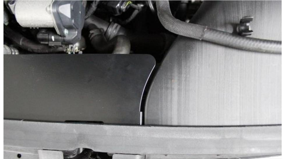
14. Adjust the height of the top panel so it sits level with the duct and then tighten the screw you used to put them together in step 9.
