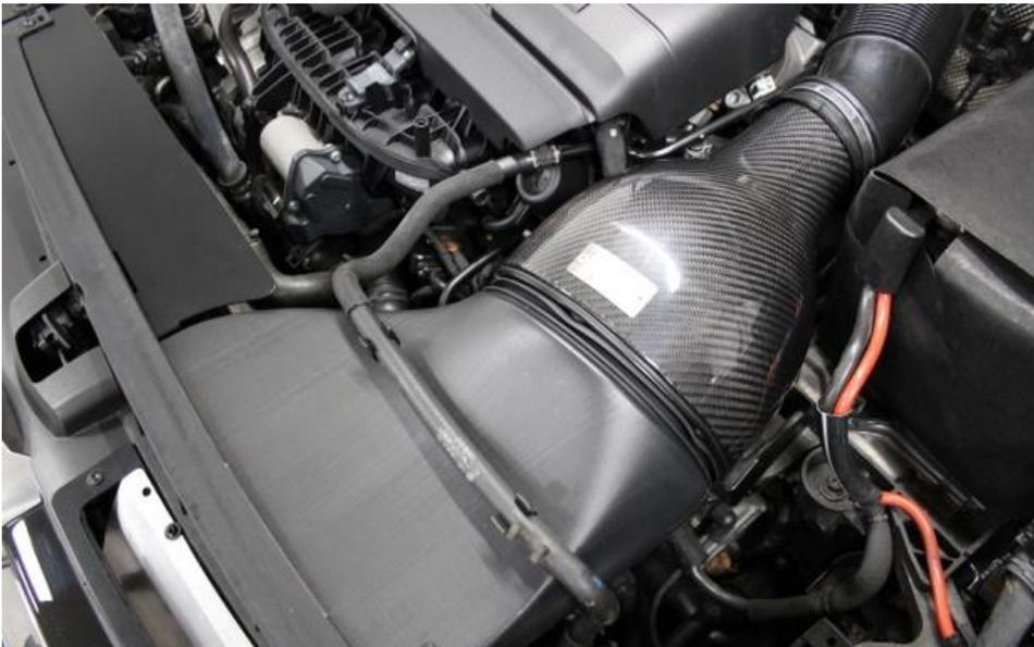
19. Lower the housing so that it locates inside the duct as shown. The rubber seal should be evenly compressed.
