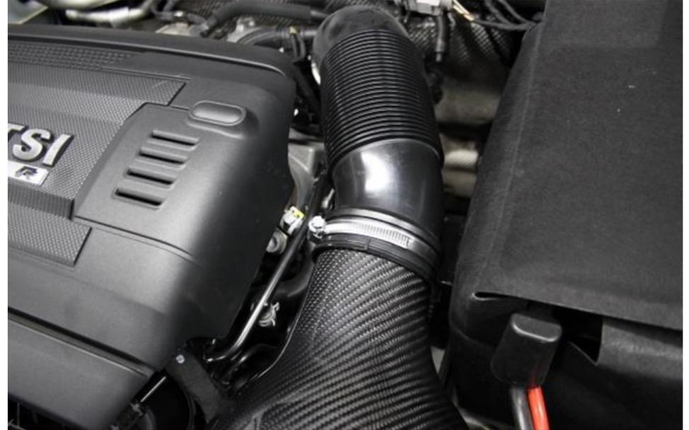
22. Tighten the hose clamp around the filter housing.
