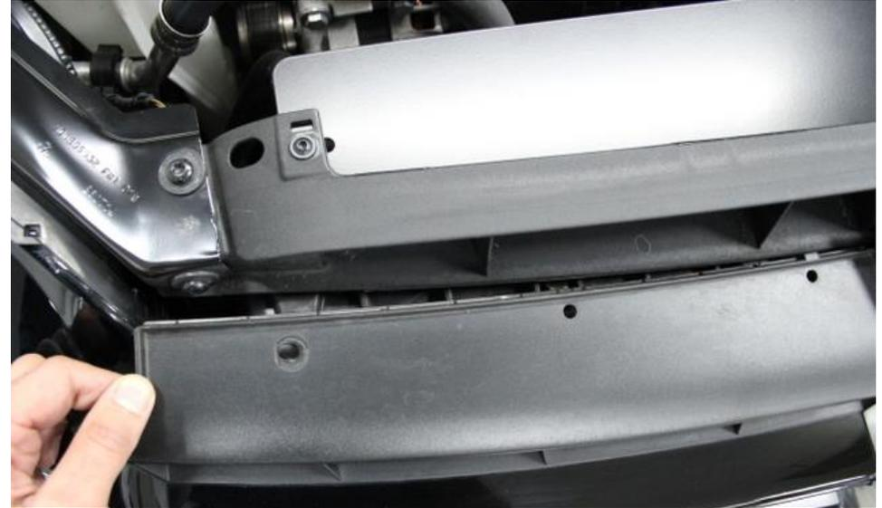
24. Once both screws are removed, carefully pull the top of the grill away from the slam panel.
