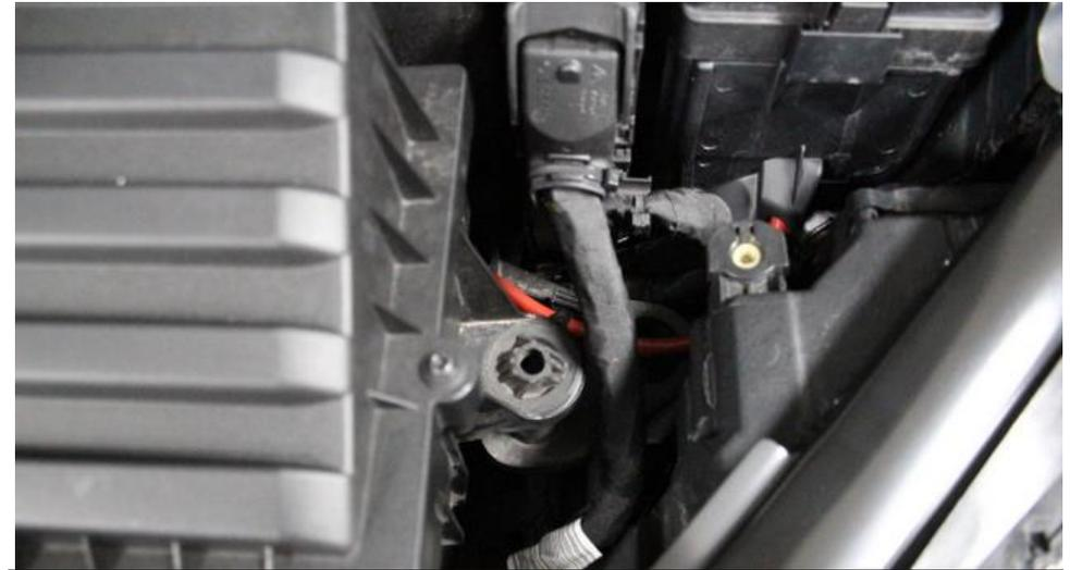
6. The airbox is held in place with some rubber mounts. Pull the airbox upwards to release from the mounts and remove from engine bay. There is also a vacuum/boost tube attached to the side of the airbox (engine side) – remove this tube by pulling it before removing the airbox.
