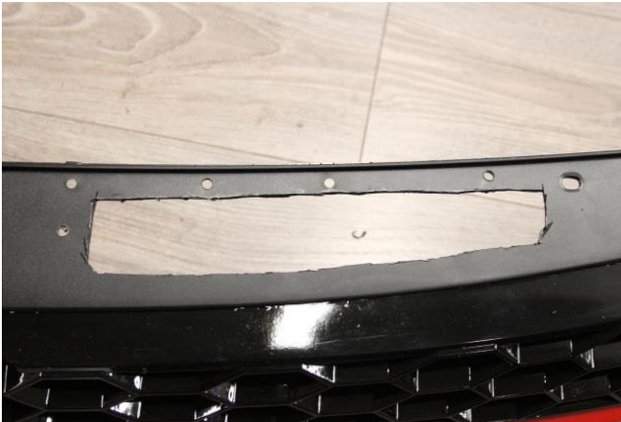
30. Use the tool in a rotary tool or a drill and carefully cut around the lines previously drawn on the grill. USE SAFETY GOGGLES when cutting. The cut does not need to be very neat since it will be covered by the scoop surround panel.
