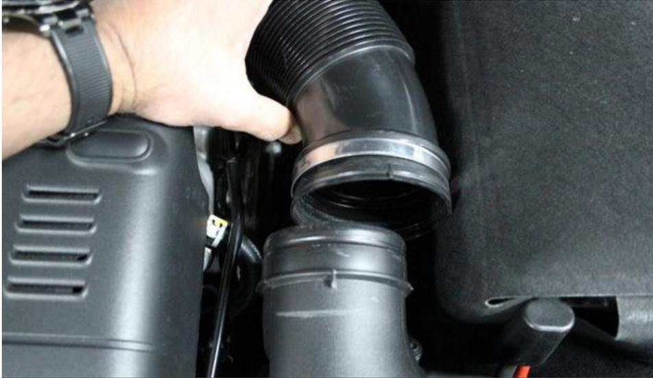
5. Compress the spring clamp around the tube and remove the tube from the airbox. Remove the clamp – we will use the new supplied hose clamp with the intake.
