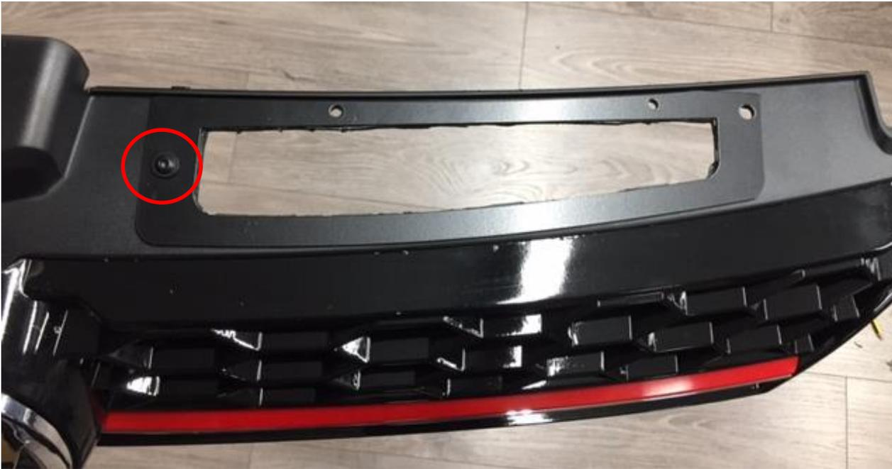
31. Place the surround panel on the grill and secure with one M5 screw and lock nut as shown. The other holes should line up. If not, drill them to line up.
