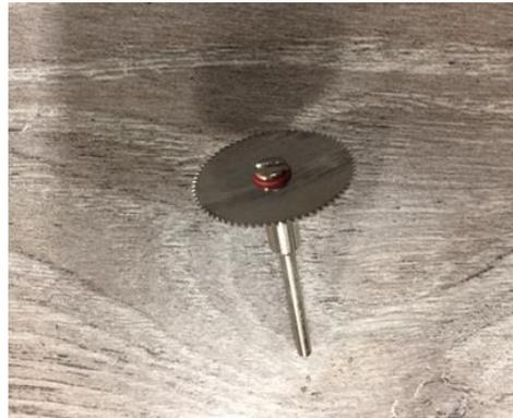
29. Now assemble the cutting disc to the shaft. Remove the screw on top of the shaft and secure it with the disc in place.
