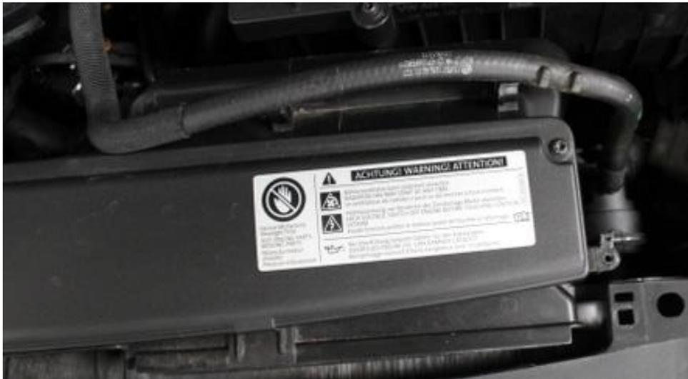
3. Now you should be able to remove the duct. If you cannot get enough movement, pull the airbox out of the mounts and push the airbox back for more clearance.
