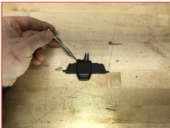
**5** **\*OPTIONAL** Use a small screwdriver to remove the directional control fork.
