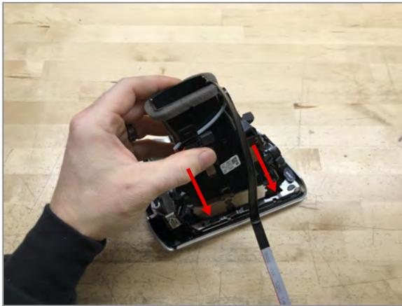
**15** Reinstall trim to vent housing, ensuring that all clips are properly seated
