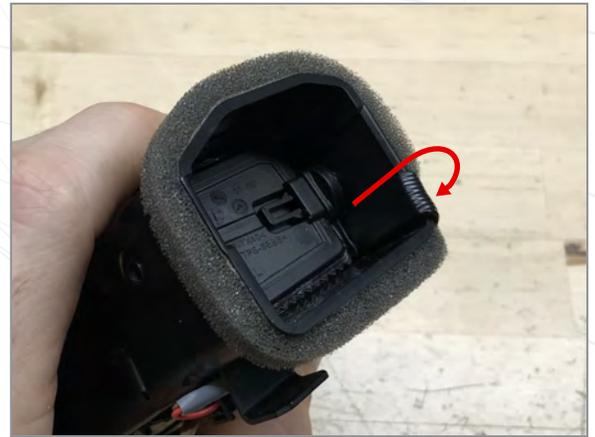
**14** Fold the display cable around the back of the vent. Close air flap to hold display cable in place during installation
