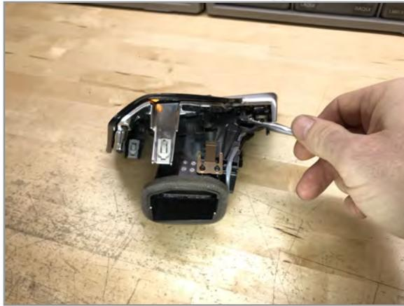
**1** Use a small screwdriver or pry tool to release vent trim clips
