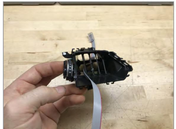
**12** Feed the display cable through the vent to the left side of the furthest left vertical slat
