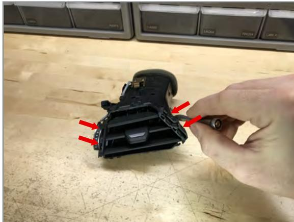
**3** Release four clips to remove vent slat assembly
