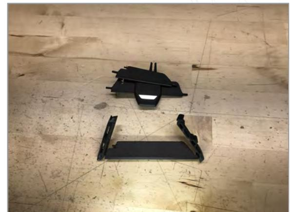
**4** Remove top two vent slats from vent assembly as shown.
