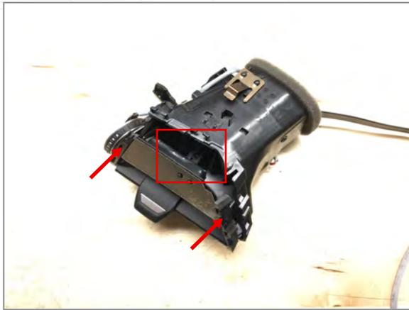
**13** If reusing slider, make sure fork extension engages proper vertical slat. Slide slat assembly into vent housing
