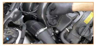
Remove the bolt that secures the remainder of the intake to the turbo. With the intake now free, remove it from the engine bay. (1x 10mm bolt)
