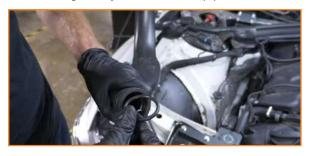
Attach a silicone coupler to the back intercooler pipe. Then set the back pipe on the turbo and slide the coupler onto the intercooler. (1x E11 torx bolt, 2x worm gear clamps)
